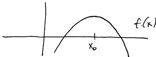
In Newton's method, you get your next guess  $x_1$  from your original guess  $x_0$  by finding where the tangent line to  $y = f(x)$  at the point  $(x_0, f(x_0))$  intersects the  $x$ -axis. Here, since the tangent line at  $(x_0, f(x_0))$  is horizontal, it never intersects the  $x$ -axis, so you can't find  $x_1$ .
